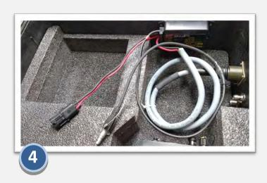
A Trimble Net R9 GPS receiver fits into the left front recess with the connections on the back of the receiver to the right side of the case. Occasionally a campaign system will be outfitted with Trimble 5700 or R7 receiver. For these situations, the setup will be the same.
