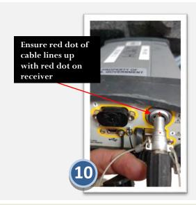
The long coaxial cable provided in the case will extend from the external TNC antenna bulkhead connection to the GPS antenna. Install the antenna on your monument *before* connecting the cable. Be careful to not kink the cable or get snow, water, dirt etc. in the cable connection to ensure good cable transmission and quality data.
