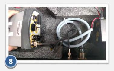
The antenna connection to the receiver passes through a TNC bulkhead installed on the front case wall. Use the small (~50cm long) coaxial antenna cable to connect the GPS receiver to the TNC bulkhead. Please be mindful to not cross thread the connections.
