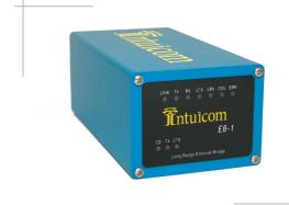
Intuicom's EB-1 Ethernet Bridge is a high performance Ethernet data transceiver designed for long range communications in commercial, industrial, and military applications. Providing wireless bridging of remote Ethernet devices, the EB-1 is ideally suited for a variety of applications ranging from basic wireless bridging to monitoring and controlling unattended systems such as those linked to SCADA terminals, automated security systems, and CBRN detection networks.
