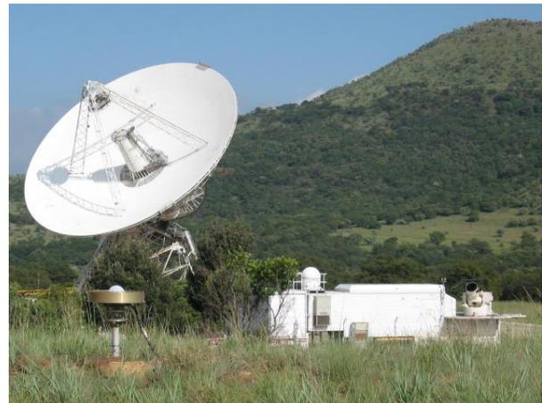
In the left foreground is a GPS antenna, in the right is the Satellite Laser Ranger and the 26 m Radio Telescope dish can be seen
