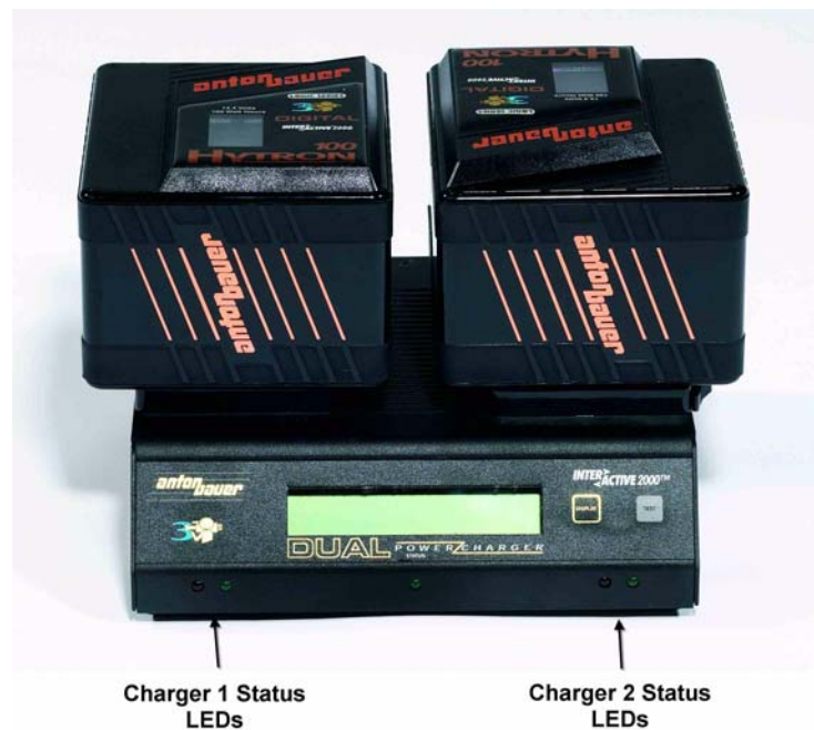
Figure 131: Battery charger with two batteries installed
