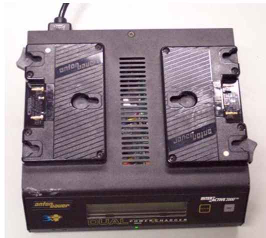
Figure 134: Battery charger, showing mounting positions and rocker switches
