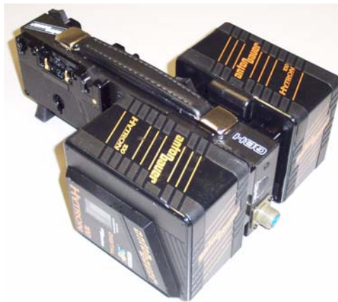
Figure 19: ILRIS-3D batteries in T-junction format
