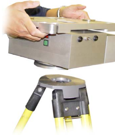
Figure 20: Mounting the pan/tilt base on top of the tripod
