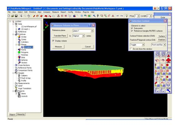
A dialogue box, as seen above, pops up on the screen. You will also see a yellow triangulated border around the solid model. These triangles extend from the edges of the data to the plane below and will be used to calculate the volume. The user then chooses the plane created earlier - in this case plane1. Click on Translate Plane to Lowest, and then click on Measure.
