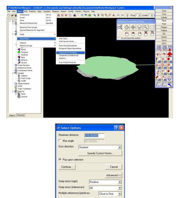
A dialogue box will pop up and the user will then select a **Maximum distance**. In this case we are using 100m to ensure that there is no data left above the plane. Clicking the advance button choose **Positive** in the **Keep errors (sign)** box. When this has been done click **Continue**.
