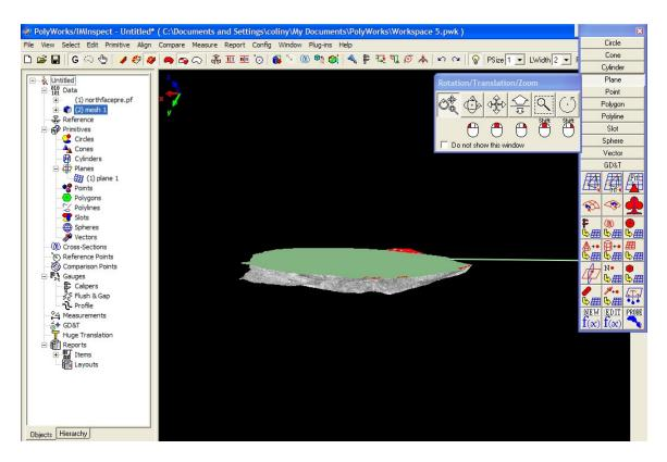
You will notice that the data below the plane has been highlighted as seen above. Clicking the delete button on the keyboard will delete the data - as seen below.
