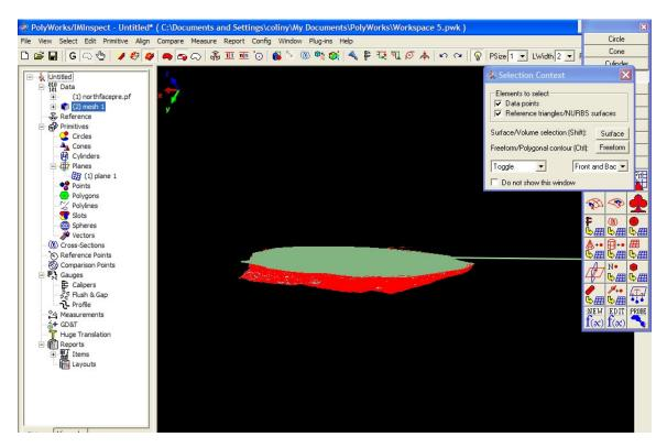
The first step in calculating the volume of the solid model is to select the stockpile as seen above, highlighted in red.
