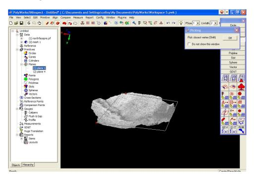
Using the rim around the pit, the user should be able to define a plane, as seen above. If the scanner operator has captured a portion of the ground around the pit, the data processing person will be able to create a plane that approximates the average elevation of the ground.
