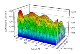
As a numerical reference, the pure elevation dependent PCV are listed below in the international ANTEX format (see ANTEX format description for details). However, the complete model of the antenna consists of elevation and azimuth dependent PCV values.
