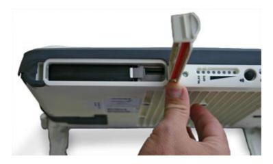
3. Push the button on the left-hand side of the SIM card holder. This releases the holder from its compartment.
