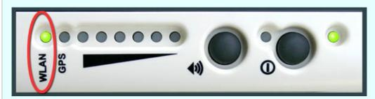
If WEP encryption is disabled, the WLAN LED lights red.
