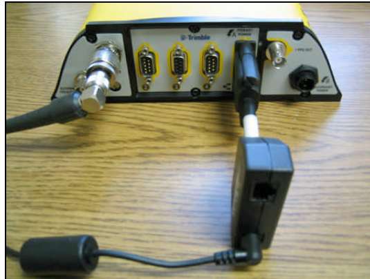
Figure 6. Back Panel Antenna and Power Connection
