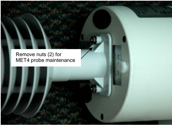
Figure 25. Gaining access to MET4 probe for maintenance
