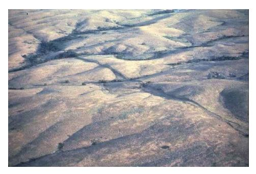
Fig. 4. The Meers Scarp in southwestern Oklahoma. It is the only visible fault scarp east of the Rocky Mountains. The scarp can be seen in this low-sun-angle air photo running from the upper left corner of the image to the lower right corner. In some places the scarp exhibits several meters of vertical offset. (Photograph by D. B. Slemmons)
