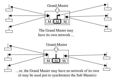
The Grand Master's network and all the Sub Masters' networks are Synchronized Networks. (The Synchronized Networks form a Synchronized System.)
