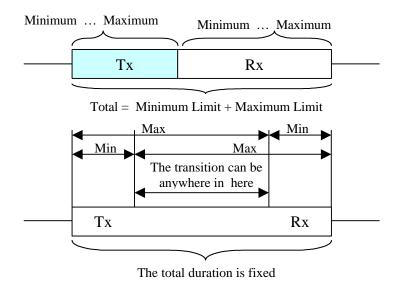
This graph shows a set of slots from a given Master at different times. This shows some of many possible combinations of bytes transmitted and received in the default settings. Note that, in addition to the bytes of data, the modems send 2 headers ( $\square$ ).
