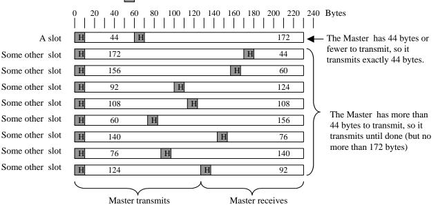
Normally you may leave these settings to their defaults. As long as no synchronized Master needs to transmit more than 44 bytes, all the Masters will transmit for exactly the same duration.
