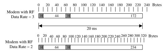
Therefore, even if some Synchronized Masters have their RF Data Rate set at '2' and some at '3', as long as they all have the same Min and Max Packet Size settings, all of them will transmit for the same duration. This would imply that networks with different RF Data Rates may be synchronized.
