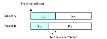
However, the length of each Master's transmission (and the point when it starts receiving) depends on how long its transmission lasts. This could result is an overlap between when one Master starts receiving and a collocated master is still transmitting; during this time, the Master that is trying to receive will be overwhelmed by the one that is still transmitting.
