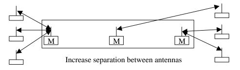
2) You must synchronize the Masters, with the Multi-Master Sync Mode. This ensures that none of the collocated Masters transmits while one of them is trying to receive.
