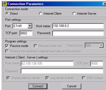
Figure 2-11. PC-CDU Connection Settings – Ethernet (Direct Example)
