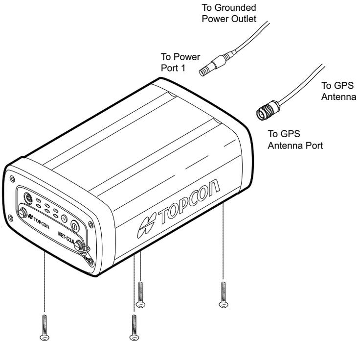
Figure 3-17. Mount Receiver and Connect Cables
