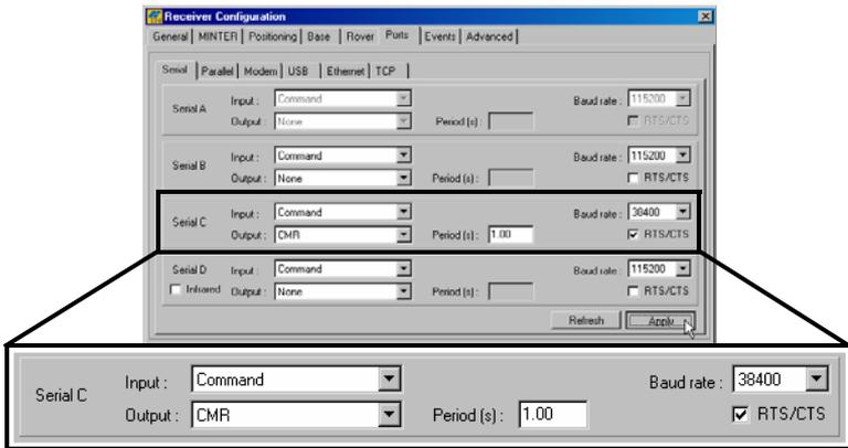
Figure 3-6. Base Configuration for RTK Surveys – Ports
