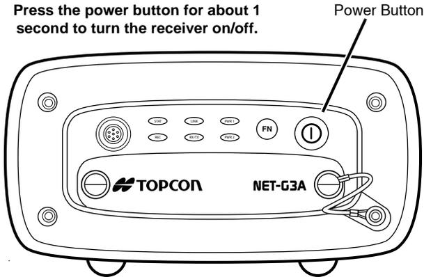
Figure 3-12. Power Button Functions
