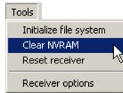
Figure 4-16. Clear NVRAM with PC-CDU
