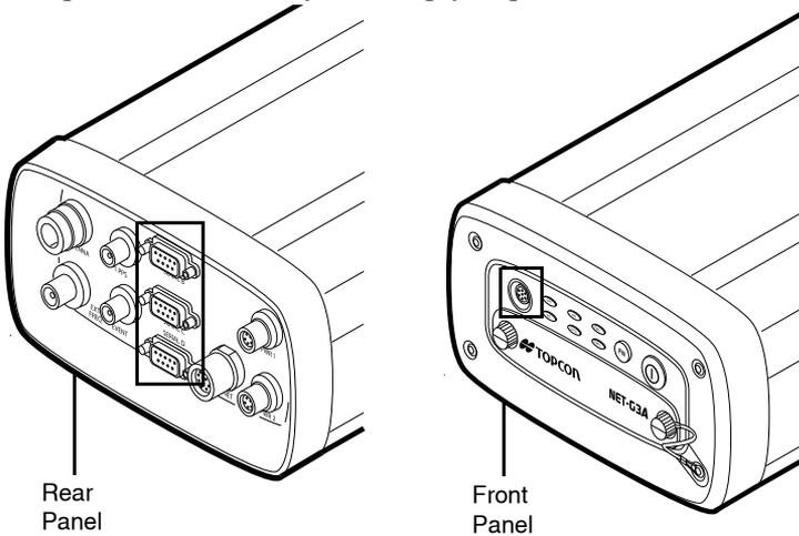
Figure 2-6. Net-G3A Serial Ports
