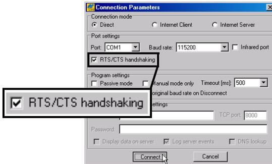
Figure 4-5. Connection Parameters – RTS/CTS Handshaking
