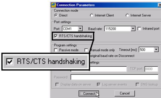
Figure 4-1. Connection Parameters – RTS/CTS Handshaking
