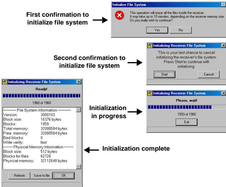
Figure 4-12. Initializing the File System
