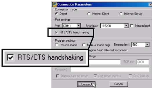
Figure 3-9. Connection Parameters – MINTER Settings
