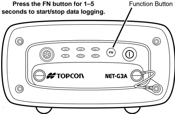
Figure 3-13. FN Button Functions
