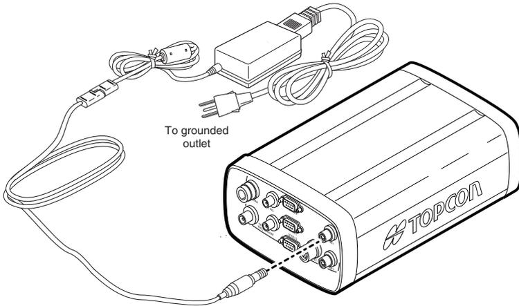
Figure 2-5. Connecting the Net-G3 to a Power Source
