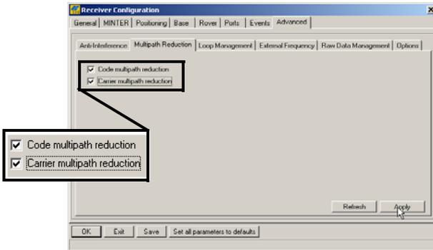
Figure 3-7. Configure Multipath Parameters
