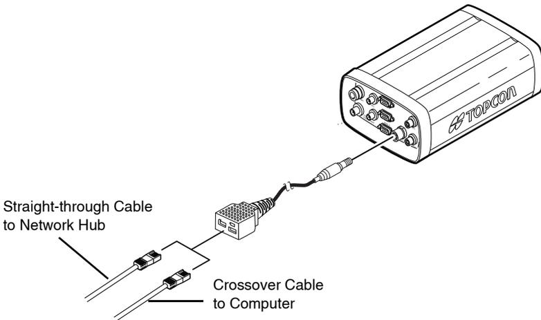
**Figure 2-8. Connect Ethernet Cable**
