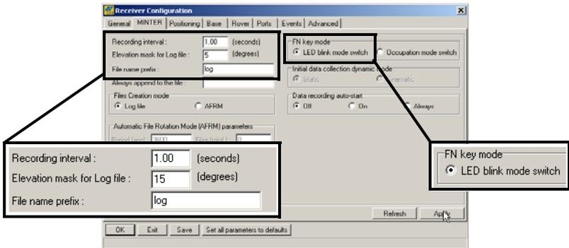
Figure 3-3. Configure MINTER for Static Data Recording
