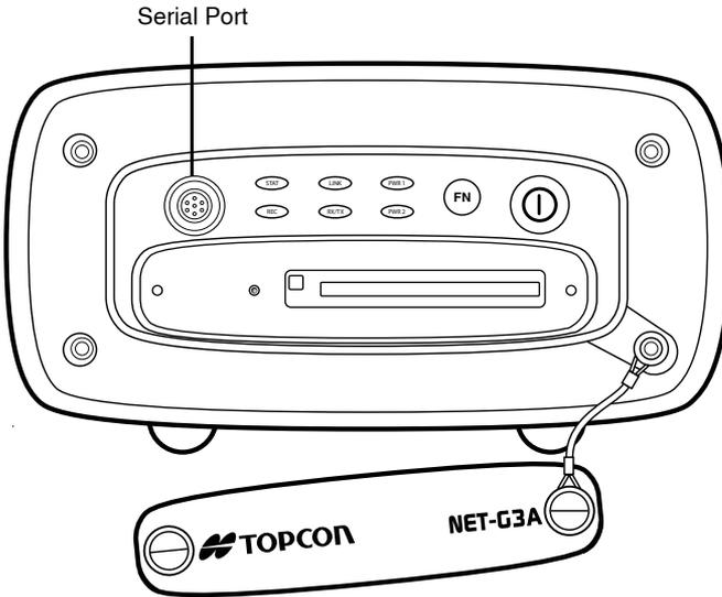
Figure 1-3. Net-G3A Front Panel Ports
