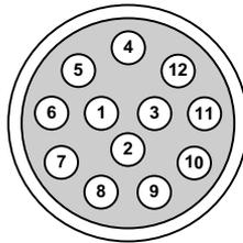
**Figure A-5. Ethernet Connector**
