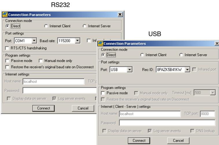
**Figure 2-10. PC-CDU Connection Settings – RS232 and USB**
