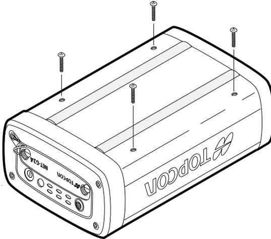
Figure 1-7. Net-G3A Bottom Mounting Holes
