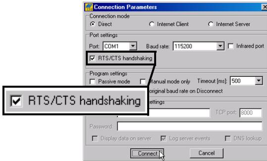
**Figure 4-10. Connection Parameters – RTS/CTS Handshaking**
