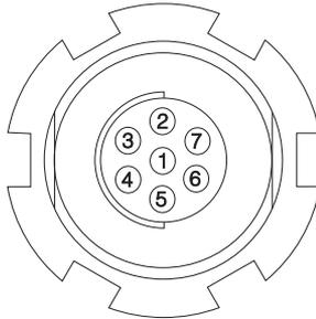
Figure A-3. Serial RS232 Connector
