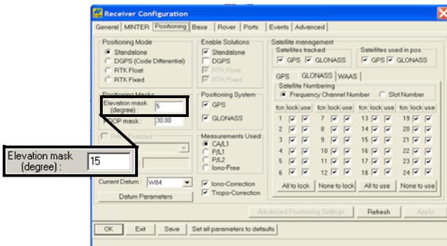
Figure 3-4. Configure Receiver Positioning – Elevation Mask
