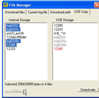
Figure 4-8. Copying Data Files to a UMS device
