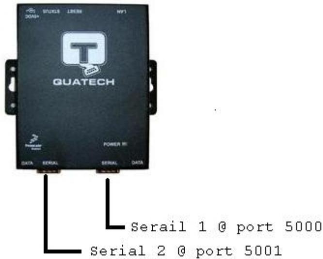
Now, suppose the IP address to the Serial Server is 69.44.87.150 and you have a MicroZ attached to Serial 1, then to create a virtual serial port on your pc to communicate with the MicroZ you would run
