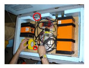
14. Connect Q330 power cable (Q330 POWER) to POWER port on seismic logger (Q330)
