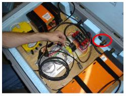
11. Connect geophone bulkhead cable (SEISMIC SENSOR) to SENSOR A port on seismic logger (Q330).
