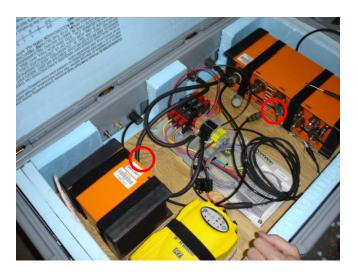
16. Connect GPS power cable (GPS POWER) to port 2 or 3 on the GPS Reciver (R7). Make sure to line red dots up before pressing in.
