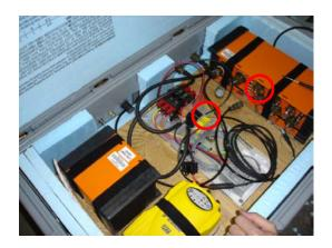
15. Connect Quet cable (shipped in PASCAL HARDIGG) to Quet port on the seismic logger (Q330) and the Quet Serial port on the bailer. Cable is symmetric.
