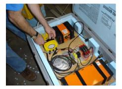
9. Attach SOLAR bulkhead cable end (bare wires) to circuit board. White end goes into orange (SOLAR) screw terminal, Black end into goes into black (GROUND) screw terminal.
