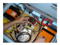
10. Attach camera bulkhead cable end (bare wires) to circuit boards. White end goes into yellow (LOAD) screw terminal, Black end into black (GROUND) screw terminal.
