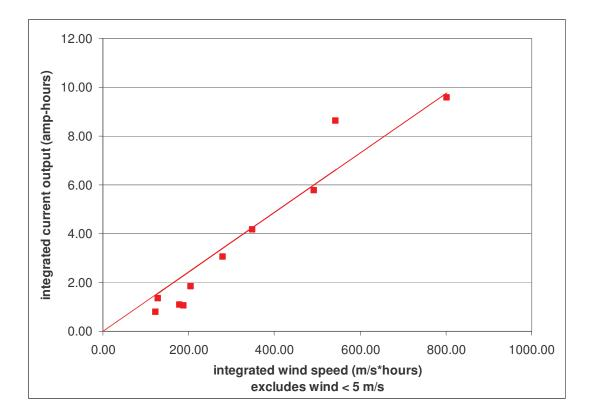
Figure 2. Using Wind Speed Data to Predict Forgen 500 Output
