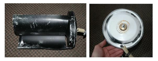
Figure 3. Forgen 500 Turbine Damage After Winter at Minna Bluff Antarctica.
