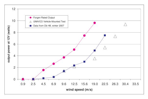
Figure 1. Forgen 500 output power at 12V.
