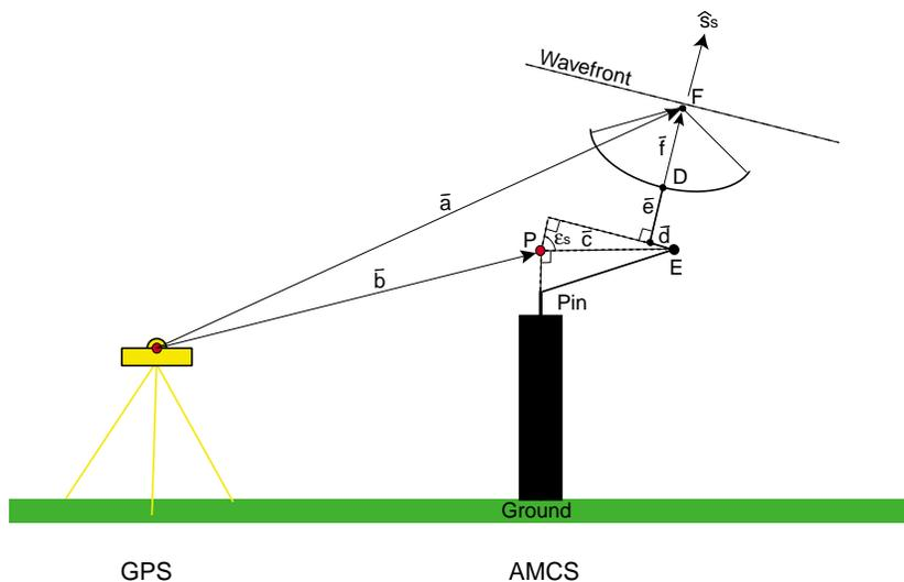
**Figure 2** Schematic representation of the geometry of the AMCS baseline model; perfect pointing.
