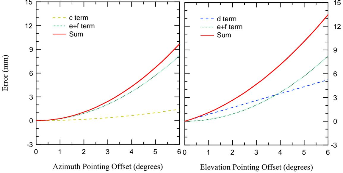
**Figure 4** Mispointing error after (7) for (left)  $\Delta\varepsilon$  and  $\varepsilon_s = 0^\circ$ , and (right)  $\Delta\phi = 0^\circ$ .
