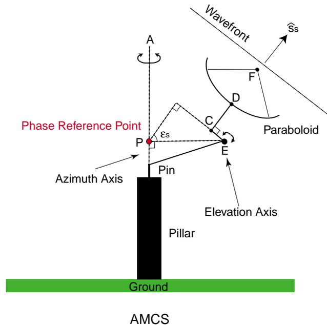
**Figure 1** Schematic representation of the (not to scale) geometry of the AMCS antenna model.
