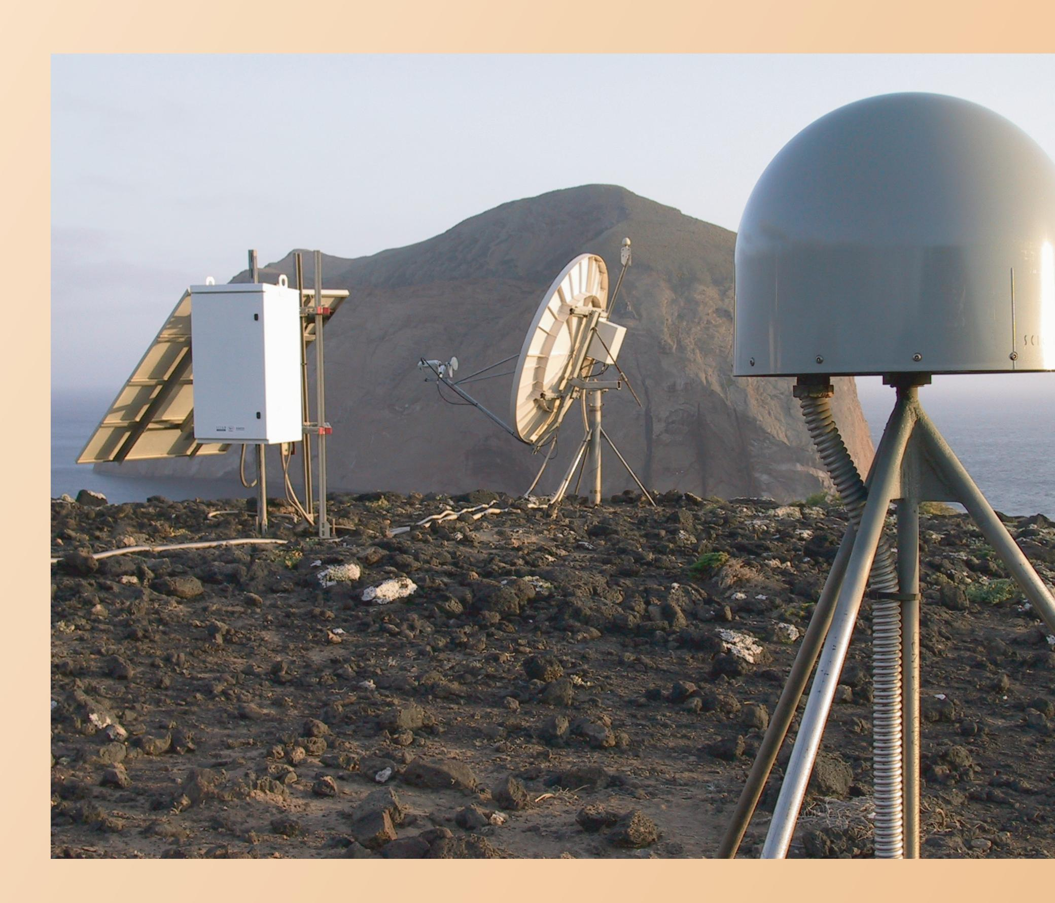
Isla Guadelupe is within the Pacific Plate, and clearly outboard of the continental crust of the borderland. CICESE, UNAVCO and SCIGN collaborated to install a GPS station whose data are being acquired through a state of the art 'VSAT' satellite telemetry system.<sup>28</sup>
