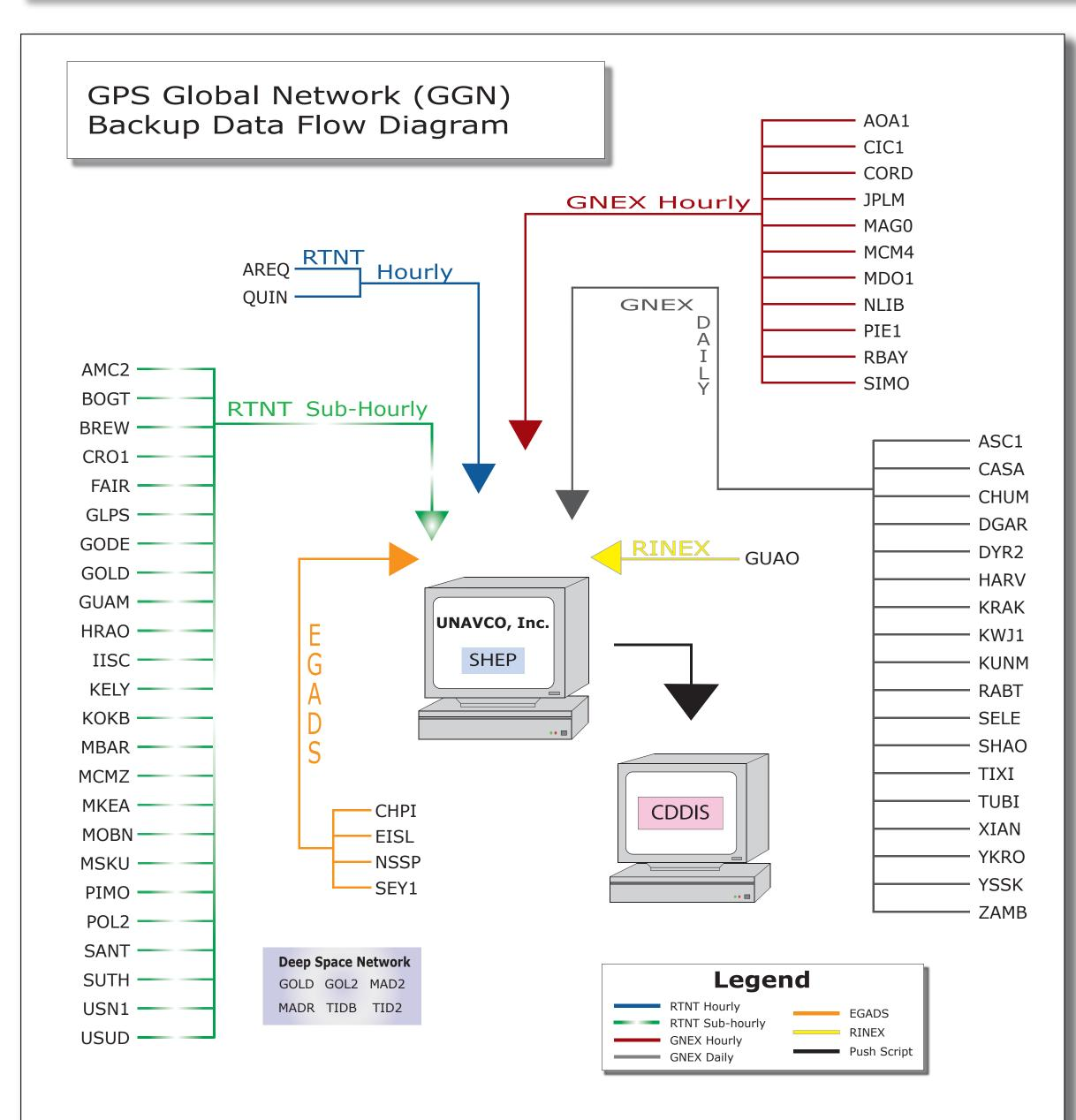
Schematic representation of UNAVCO backup operations of JPL data transfers. UNAVCO maintains a continuous readiness to provide data backup of JPL functions in case of an outage in JPL operations. The backup functions include data retrieval, RINEX conversion, data archiving, and data forwarding to the CDDIS of regular IGS products. In addition, normal station troubleshooting and maintenance tasks are provided during outages.
