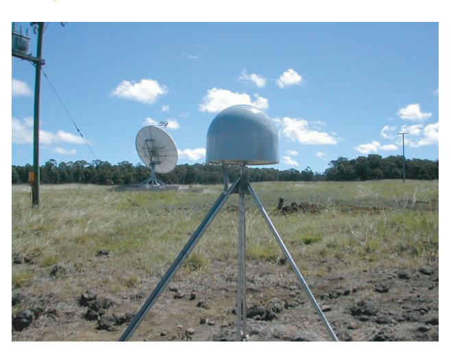
The newly erected SCIGN stainless steel, short drill-braced monument on Easter Island (ISPA). The new station runs an Ashtech MicroZ receiver with Ashtech Choke Ring Antenna and Tall SCIGN Radome. The station also includes a MET pack for meteorological measurements. Station uses a Linux computer and shares VSAT data communications routing with IRIS Seismic station.
