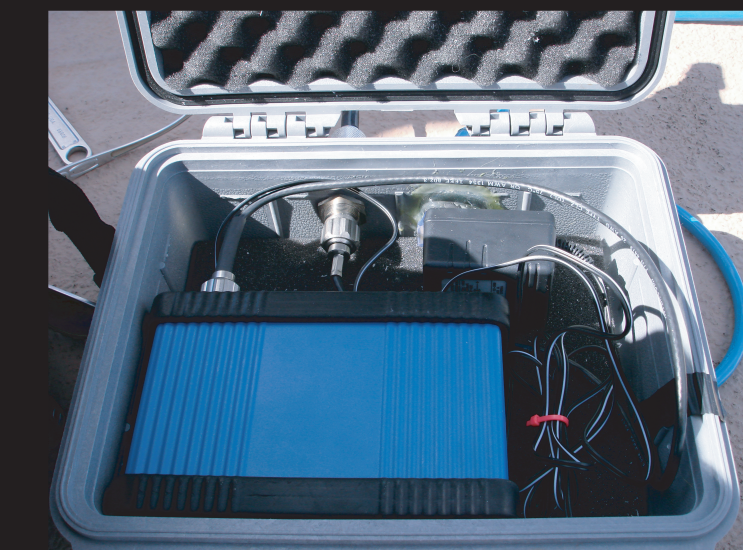
Box that houses repeater up at NCAR for Marshall field wireless ethernet connection.
