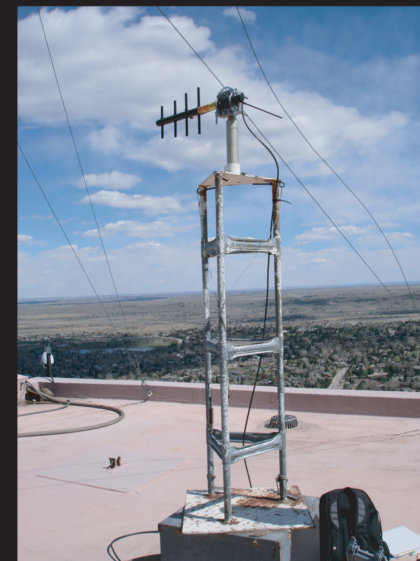
Yagi directional antenna connected to repeater used for communication to Marshall field test site.
