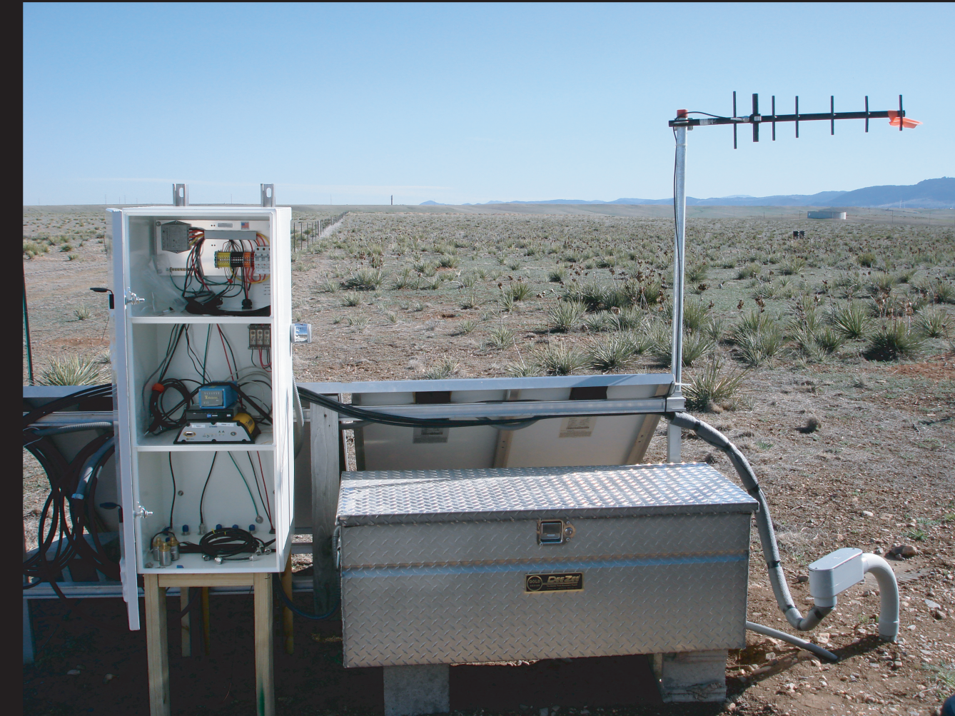
Marshall Field Test Site near Boulder, Colorado, uses a pair of wireless ethernet bridges which communicate through a repeater located up at the National Center for Atmospheric Research (NCAR).
