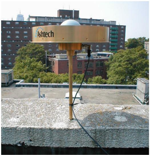
Detail of ground installation. This test case was not installed that well (drilled into surface crack and the concrete was coarse grained.
