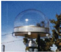
Figure 10: Picture of UNAVCO dome mounted on a Trimble Dorne Margolin choke ring antenna
