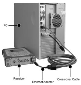
Figure 1-8. Direct Ethernet Connection – Hardware Setup
