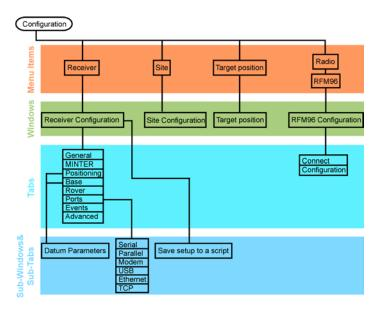
Figure 3-5. Configuration Menu Structure
