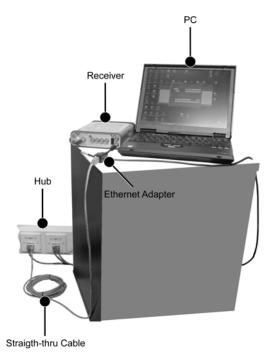
Figure 1-11. Receiver on LAN - Hardware Setup
