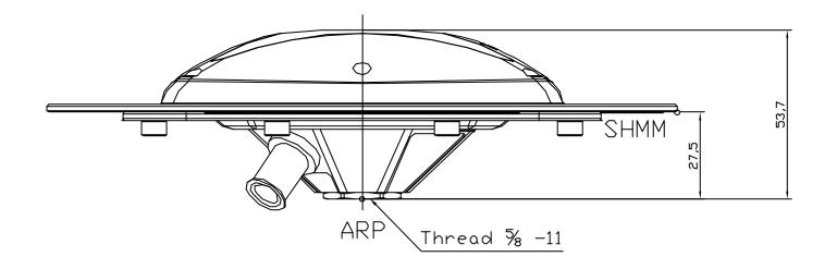
Dimensions are in mm ARP - Antenna Reference Point SHMM - Slant Height Measure Mark
